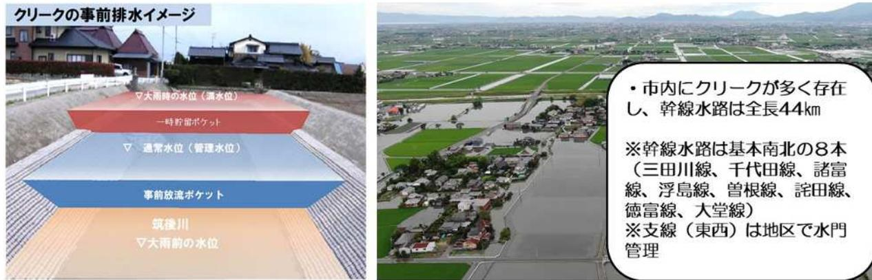
The diagram on the left shows a cross-section of a creek with several levels: '大雨時の水位(湛水位)' (Water level during heavy rain), '一時貯留ポケット' (Temporary storage pocket), '通常水位(管理水位)' (Normal water level), '事前放流ポケット' (Pre-release pocket), and '筑後川' (Kikugawa). The aerial view on the right shows the creek flowing through a residential area with green fields.
