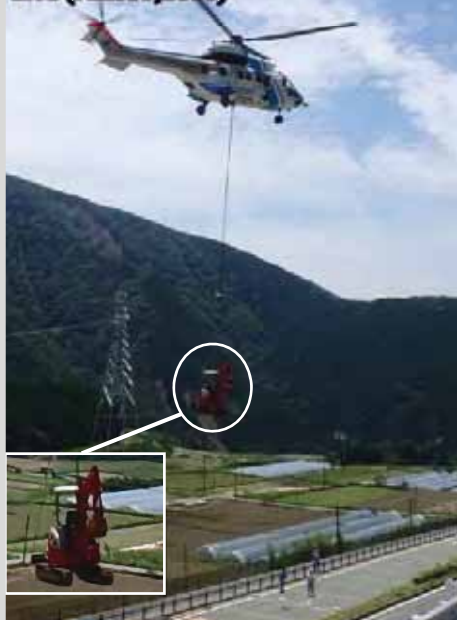
Transporting construction machinery to the upper part of the Aso mountain area (June18,2016)
