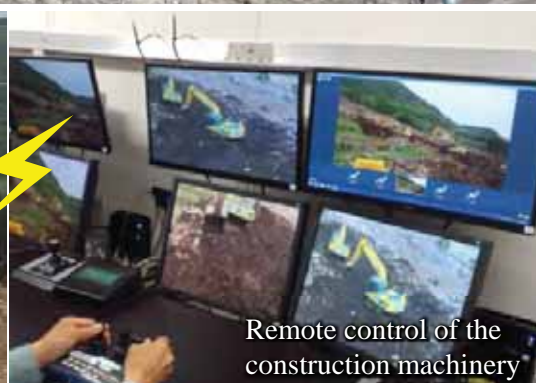
The unmanned construction machinery in action (June11,2016)
