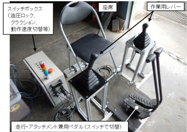
図-16 操縦席型操作器
